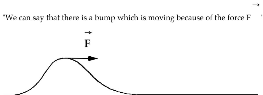
The force is localized only on the bump and has the same direction as the propagation velocity. The velocity and the force seem to have been combined.
